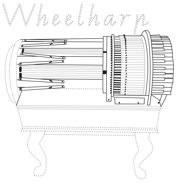
Has a keyboard and foot controlled motor.
